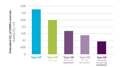
The chart to the left shows a comparison of embodied carbon in various concrete mixes.
