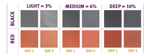
The above table is provided as a guide to illustrate the difference in colour saturation of both the ratio of oxide (Light, Medium or Deep) to cement, as well as colour lightening over the first 5 days as the cement cures. Ensure your ratio percentage is based on the cement content only, as oxide will not colour sand or stone.
